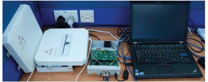
Fig. 4. Testbed: Two circular antennas are mounted to USRP N210. The USRP N210 is connected via GigE to a laptop that acts as an RFID reader.
