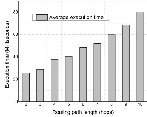
Fig. 18. Program execution time of compressive-sensing-based path reconstruction by CSRP versus the routing path length.
