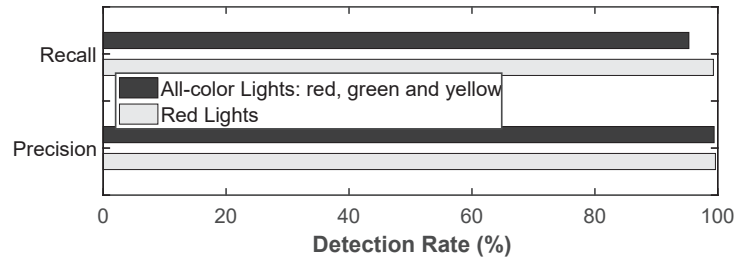
Fig. 15. Precision and recall of the traffic light detection. We compare the detection for red light only and the detection for all three lights together.
